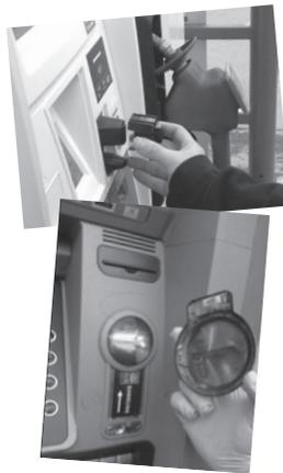
We want you to be aware that ATM/Gas Pump skimming/shimming devices have been on the rise in our area. Although we have not had any issues with our ATM machines, some of our members have recently had fraudulent debit transactions. Thieves are installing these types of devices on local ATM and Gas Pump card readers to capture your card information. Once they have your card information, they are able to make fake cards to make purchases or withdrawals from your account.
